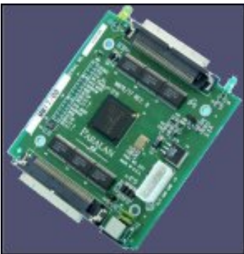
The board-level version Model MM17 is sized to fit in a standard 5.25" drive bay.
